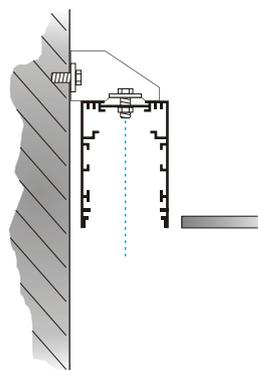
Ceiling cut-out to be produced on-site by the ceiling builder. Ceiling finished with finishing profile.
