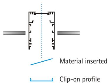
Ceiling cut-out produced very exactly on-site using solid ceiling plaster profiles.
