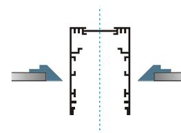
Using individually precast, shaped plaster parts produces a unified appearance of the ceiling system and luminaire. The shaped plaster parts are designed to fit the luminaires to be installed, ensuring uncomplicated installation by the specialist fitters. The variety of shapes is limitless, giving
