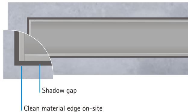
Wall-mounting the luminaire with wall bracket with predefined offset from wall. Fitting to the ceiling with joint. Ceiling finished with finishing profile.
