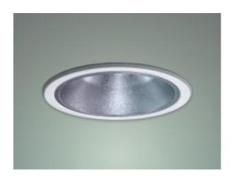
SOBRA recessed downlight equipped for general service lamps and high-pressure discharge lamps with E27 lampholder. Vertical burning position. Aluminium reflector, polished and piece silver anodized.
