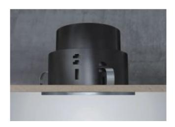
Three-piece luminaire housing consisting of a mounting frame with mounting system, luminaire housing and crisp-edged cover ring with fixing screws.
