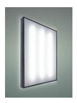
Equipped for T5 fluorescent lamps or compact fluorescent lamps. With electronic control gear, AC/DC. Also available as dimmable MultiPower version with DALI or 1–10V interface. Prewired and ready for installation with heat resistant cable and terminal block for through wiring, 3–pole (5–pole). Luminaire suitable as emergency light. Installation of specific emergency-light components such as monitoring parts and single batteries is possible.
