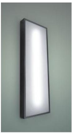
Equipped for T5 fluorescent lamps or compact fluorescent lamps. With electronic control gear, AC/DC. Also available as dimmable MultiPower version with DALI or 1–10V interface. Prewired and ready for installation with heat resistant cable and terminal block for through wiring, 3–pole (5–pole). Luminaire suitable as emergency light. Installation of specific emergency-light components such as monitoring parts and single batteries is possible.
