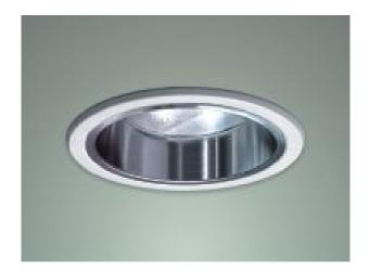
SOBRA recessed downlight equipped for CDM-T high-pressure discharge lamps. Horizontal burning position. Luminaire with electronic control gear, non-regulable, in separate housing.
