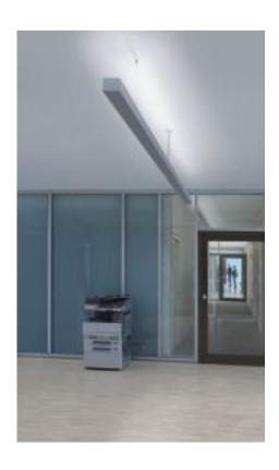
Sharp-edged, drawn aluminium profile with minimum dimensions. One-piece housing with just two suspension points. The electronic control gear is integrated in the blank constructional elements. Mounting as pendant luminaire with wirerope rapid connector system.
