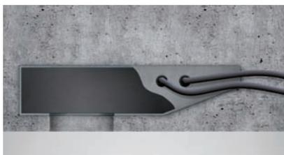
► The trimless installation in cast concrete ceilings can be realised using specially developed cast-in housings. The use of a variable core element means this is also possible with bare concrete ceilings.
