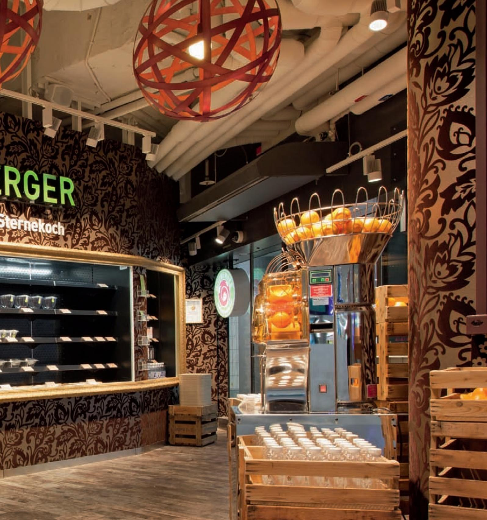
previously used halogen spots. Lighting situations for the seasonally changing product spectrum can be adapted thanks to flexible positioning of the luminaires along the track and the possibility of exchanging reflectors without tools. Despite the ceiling being already overloaded with building service installations, the lighting designers aimed for a flexible lighting concept, and tracks
